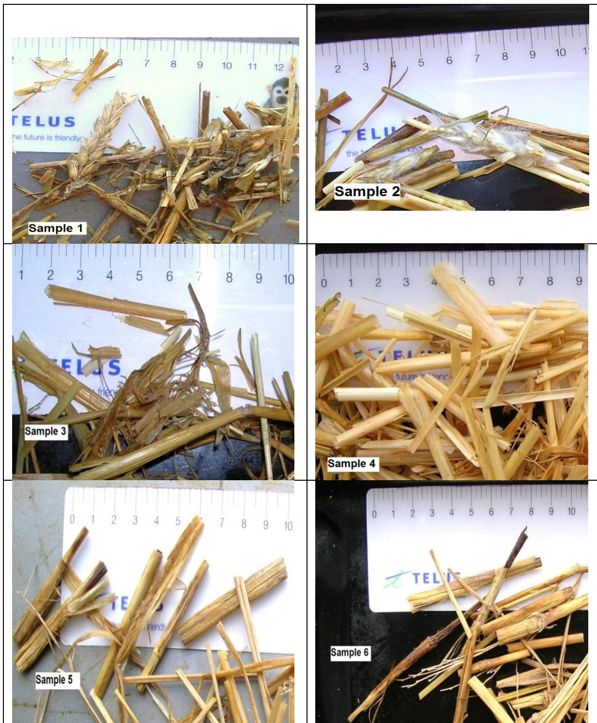
Figure 14: Photographs of samples once experiments were complete (white growth particularly apparent on sample 2 and dark growth on samples 5 & 6.
